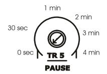
Dip switches DS1: 1 to 3 need to be set for an operating mode with PAUSE time for this adjustment to have any effect
